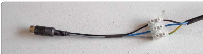
Photo 6: Terminal block to 5 pin DIN connector.
